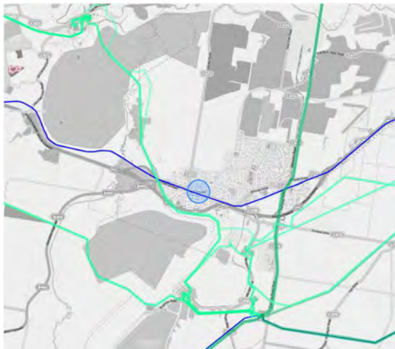
Figure 22 VicTrack fibre and power transmission network around Morwell
